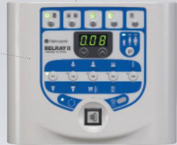
Control panel can be mounted outside of the X-Ray room with a hand exposure switch for remote control
